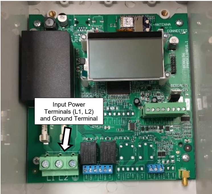
Figure 4 – Input Power Terminal Locations
